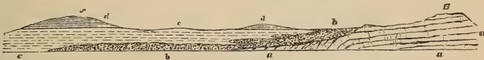
FIG. 211.—SECTION NEAR BRISTOL TO SHOW HOW CONGLOMERATE MAY PASS INTO CLAY ALONG THE SAME HORIZON.
